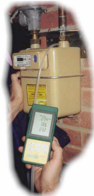
After the test period has been achieved, press and hold “**Light**” again to clear the alternating display of “**P1**” and the “dropped” pressure reading. A solid “**P2**” is displayed at the bottom of the screen.
