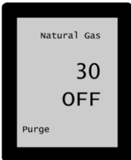
In this mode, the unit continues to pump clean air past the CO sensor. As soon as the CO level falls below 20 ppm the unit will automatically start its 30-second countdown and then turn off.
