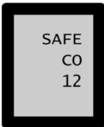
Pressing & holding the “**Log**” starts the CO room test. A reading is taken every minute for 30 minutes.
