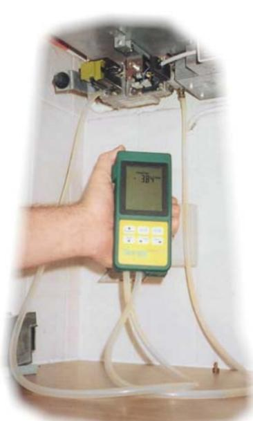
For **gauge** pressure, connect one length of silicon tubing supplied to the ‘Pressure (+)’ port (see 2.7).
